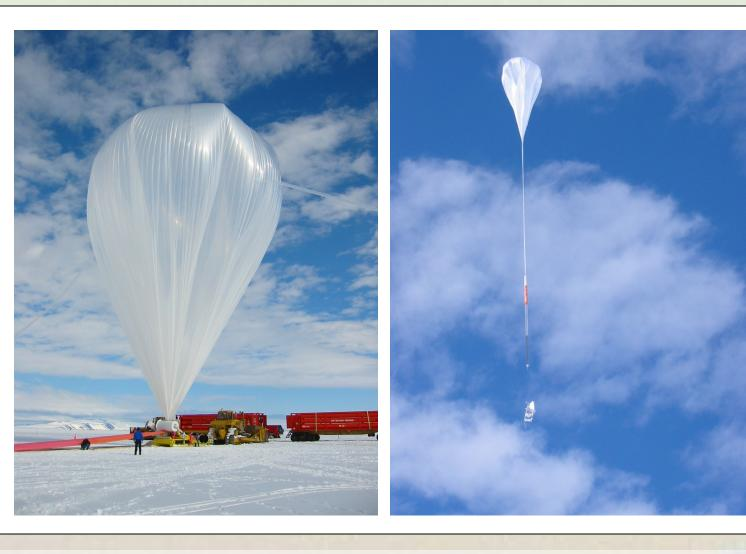
starting from 2008 the SUNRISE telescope will fly in a series of long duration balloon flights (10-14 days) over Antarctica.
